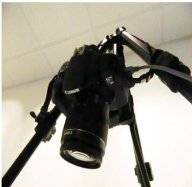
One camera that can be used is the Canon Digital single lens reflex. It connects directly to a computer running Canon's EOS software. Utilizing the computer monitor display, all the important settings can be controlled and the picture taken.
