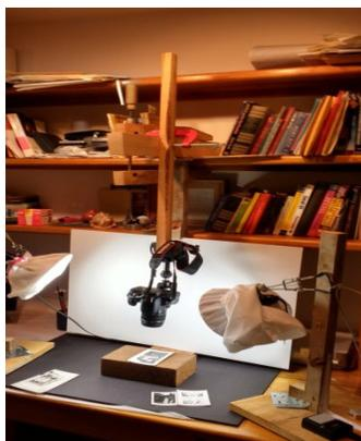
If a tripod isn't available, C clamps and a wooden beam can be clamped onto a shelf to make a home made camera mount.
